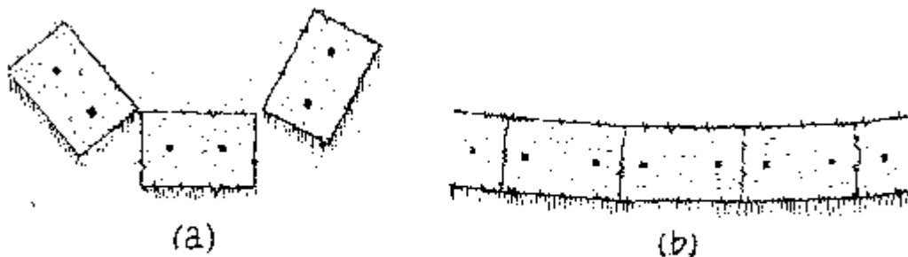
(a) INCORRECT AND (b) CORRECT ABUTMENT OF STRAW BALES IN A TRENCH
